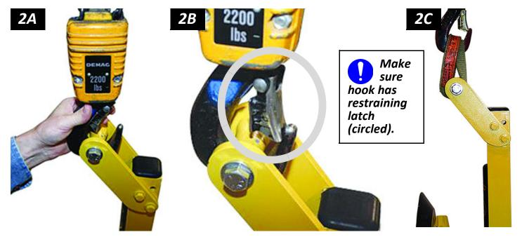
2.2) Attach the hoisting hook to the <u>lift</u> <u>point</u> (figs. 2A-B). Use rigging as
